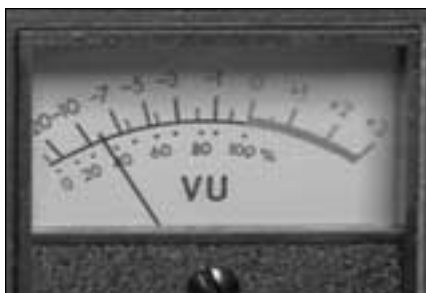
Average reading if level is set too low; may result in inadequate signal.
