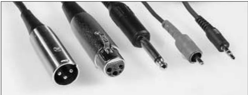
Connectors commonly used for audio (left to right): XLR (male), XLR (female), 1/4-inch phone plug, RCA or phono plug, 3.5 mm mini plug.
