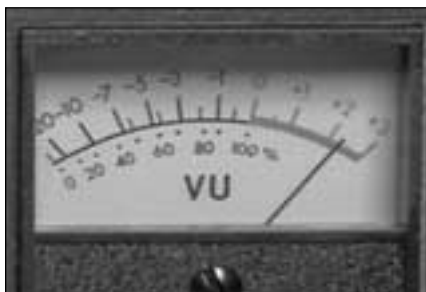
Average VU meter reading if level is set too high; may result in signal overload distortion
